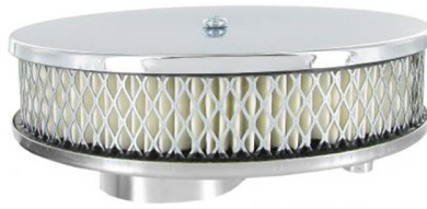
Super low air cleaner for the stock Solex carburetor Diameter: 162mm, Height: 57mm, Carburetor neck size: 51mm, Cranckcase breather connection: 13mm
