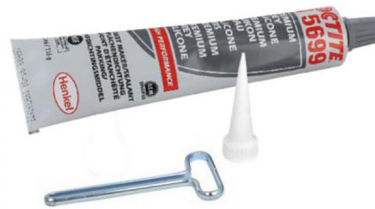
SI 5699 grey silicone sealing compound Content: 80 ml, Color: grey, Chemical Type: Oxime Silicone, Maximum sealing gap: 1.0mm, Temperature range: -60 °C to +200 °C
