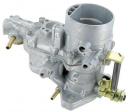
Weber 34 ICT carburetor (each) Main jet: 135, Air jet: 160, Idle jet: 55, Emulsion tube: F78
