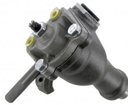
Steering box Beetle Sedan export models 1961 (4 236 757) until 7.1965, VW 1200, VW 1300 and VW 1500 8.1965 and later, Convertible 1961 (VIN 3 933 185) until 7/1970, Karmann Ghia 1961 (VIN 4 236 757) and later, Type 3 all, Thing all
